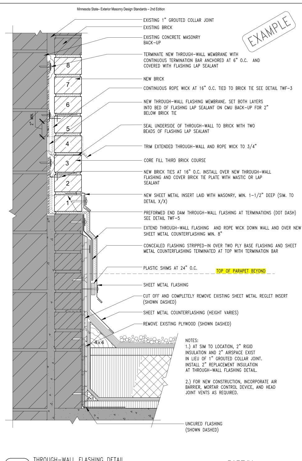
THROUGH-WALL FLASHING DETAIL WTR-1A REPAIR OR RENOVATION SCALE: 3'' = 1' - 0''
