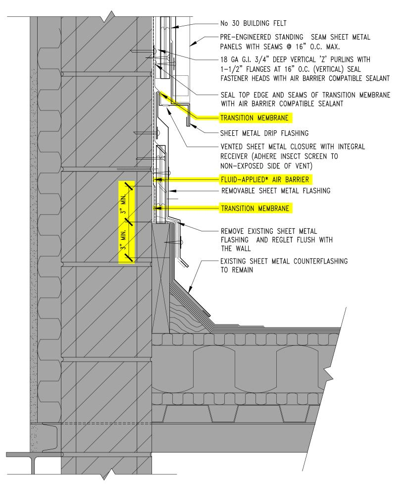
\*AIR BARRIER MEMBRANE MAYBE FLUID-APPLIED OR SELF-ADHERING.
