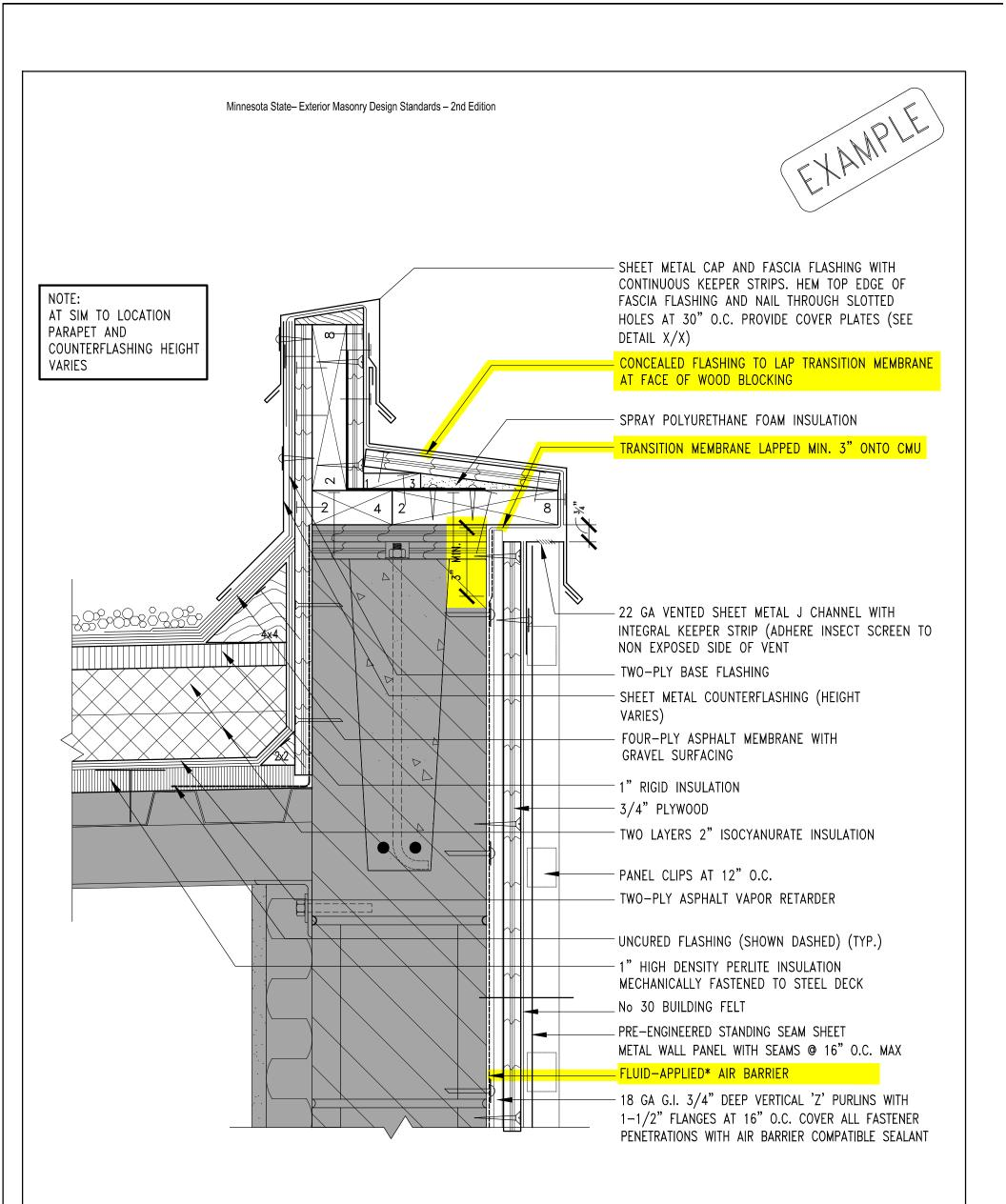
\*AIR BARRIER MEMBRANE MAYBE FLUID-APPLIED OR SELF-ADHERING.
