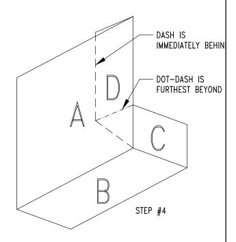
AFTER ALL FOLDS HAVE BEEN MADE. FOLD THE FLASHING AT THE 45 DEGREE BEND AND FOLD BEHIND SURFACE AREA A. THIS WILL CREATE INSIDE FOLDS BETWEEN A-B, B-C, & C-D AND AN OUTSIDE FOLD BETWEEN A-D.
